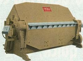
Chicago Dreis & Krump makes power leaf brakes in regular, medium and heavy duty capacities with power clamping and motorized top leaves. They're built to last, too, from their welded steel plate frames with box type supports to their powerful gear head motors with built-in magnetic brakes. So get it all, including radius bending. Box & Pan types are also available.
